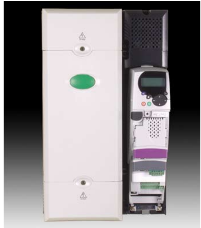
The SM-Profibus, SM-DeviceNet and SM-CANOpen Solution Modules have been fitted to this 75 hp Unidrive SP allowing it to do double duty as a communications gateway for these three fieldbus protocols.
